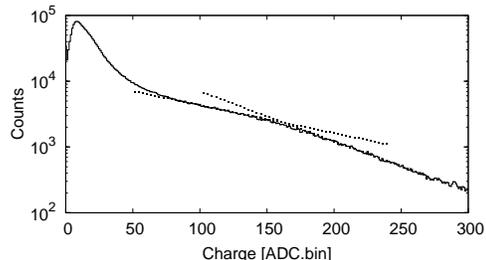
Fig. 2. Charge histogram for one minute of data of a 4 m<sup>2</sup> detector at Sierra Negra. While there is no characteristic muon peak at this altitude, a change in the slope can be determined and used for calibration. The intersection of the two fitted dotted lines is used to determine a calibration reference point.
