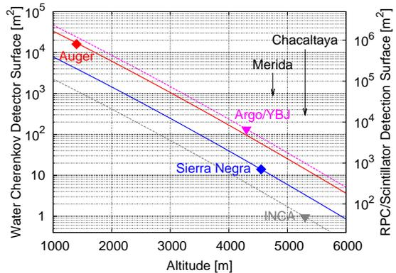
Fig. 1. Lines of equal sensitivity for experiments of different size and altitude, neglecting geolatitude cutoff and assuming similar scaler threshold. A few tens of  $m^2$  of WCD at high altitude are as efficient as currently running experiments for the SPT.
