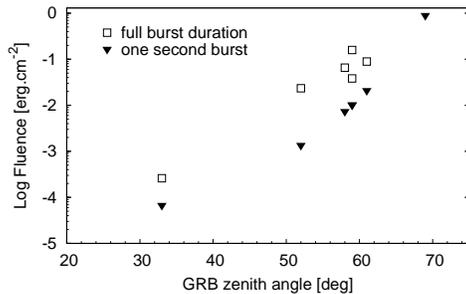
Fig. 3. 5- $\sigma$  fluence limits in the 1 GeV - 1 TeV energy range for the bursts in the field of view of Sierra Negra, for a single second burst or for a burst of same duration as detected by the satellite, assuming a spectral index of -2.
