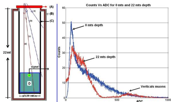
Fig. 3. In order to isolate the vertical muon flux, a WCD (D) has been installed at 22 mt depth within a reinforced (B and C) column of concrete (left). Low energy direct vertical particle has been removed with an iron filter 10 cm thick (A). A charge histogram at 0 and 22 mt depth illustrates the muon component (right).
