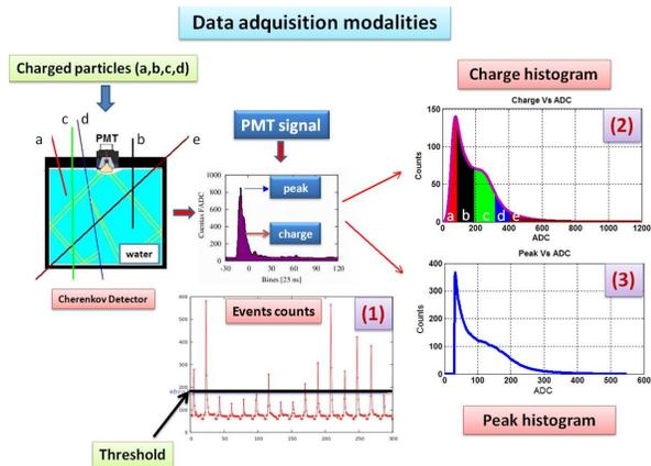
Fig. 2. High energy charged particles (a, b, c, d, e) produce Cherenkov Radiation in the water. The Cherenkov light fills the entire volume of water due to diffuse reflection on the tyvek. A light portion is collected by the PMT. The signal can be acquired as single events (1), charge (2) or peak histogram (3).
